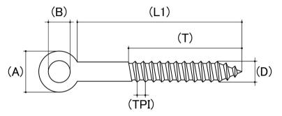
Lag Eye Screw Material: Stainless Steel Class Grade: A4-70 G316 Corrosion Protection Level: Ultimate
